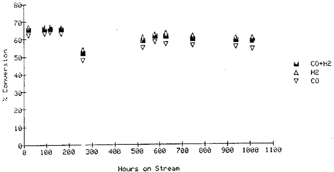
Figure IX.11. Conversion maintenance - extended slurry test 8862-1-31 Co/Zr/SiO<sub>2</sub>, 240°C, CO/H<sub>2</sub> = 0.5, 1.8 L/g/hr, 300 psig.
