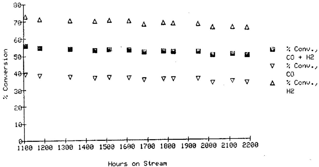
Figure IX.13. Conversion maintenance - extended slurry test 8862-1-31 (Co/Zr/SiO<sub>2</sub>, 260°C, CO/H<sub>2</sub> = 1.0, 2.0 NL/g/hr, 300 psig).
