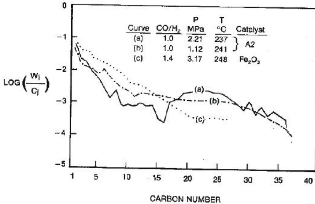
Figure IX.8. Hydrocarbon Schulz-Flory distribution of slurry catalyst A2.
