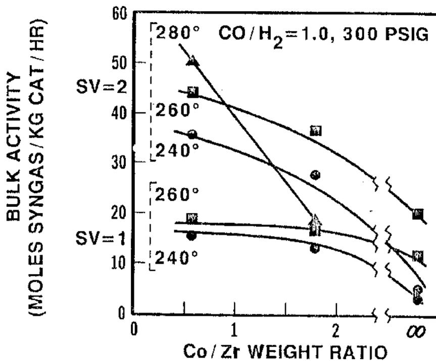
Figure IX.5. Effect of Co/Zr weight ratio on slurry-phase activity of Co/Zr/silica catalysts.
