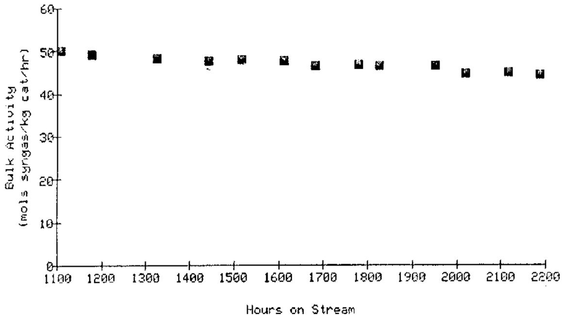
Figure IX.12. Bulk activity maintenance - extended slurry test 8862-1-31 (Co/Zr/SiO<sub>2</sub>, 260°C, CO/H<sub>2</sub> = 1.0, 2.0 NL/g/hr, 300 psig).
