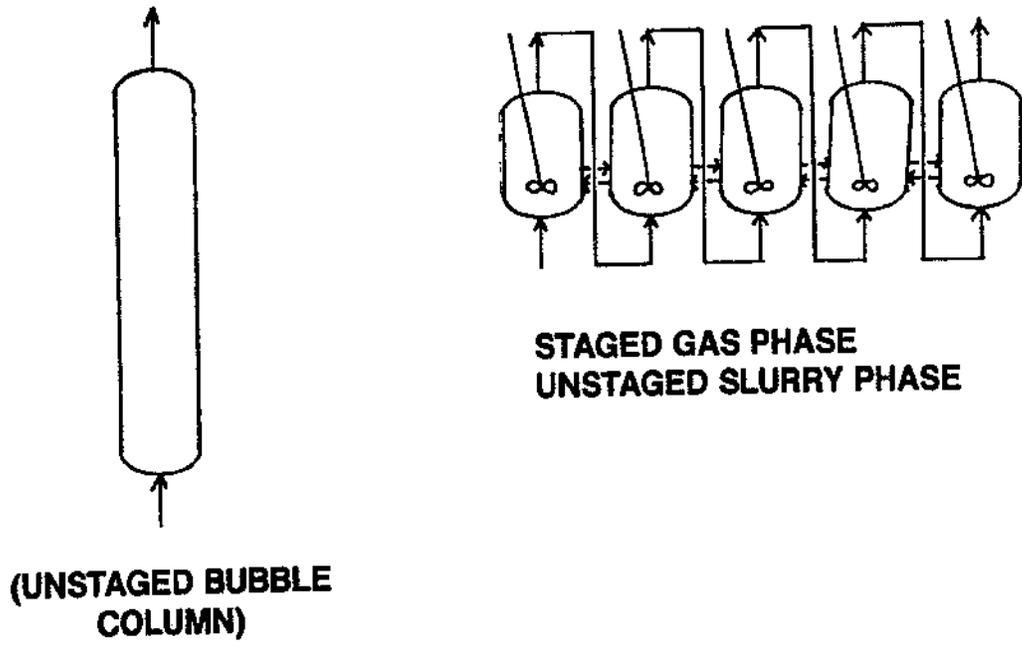
Figure IX.18. Staged reaction systems.
