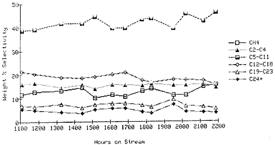
Figure IX.14. Hydrocarbon selectivity — extended slurry test 8862-1-31 (Co/Zr/SiO<sub>2</sub>, 260°C, CO/H<sub>2</sub> = 1.0, 2.0 NL/g/hr, 300 psig).
