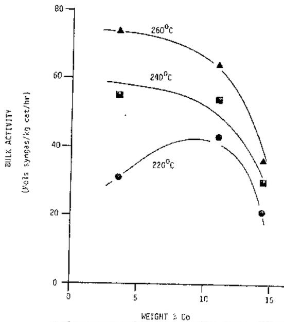
Figure IX.6. Effect of cobalt loading on bulk activity of Co/Zr/SiO<sub>2</sub> Catalyst (fixed bed reactor, CO/H<sub>2</sub> = 1, 1000 hr<sup>-1</sup>, 300 psig).
