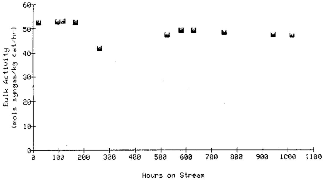
Figure IX.10. Bulk activity maintenance - extended slurry test 8862-1-31 Co/Zr/SiO<sub>2</sub>, 240°C, CO/H<sub>2</sub> = 0.5, 1.8 L/g/hr, 300 psig.
